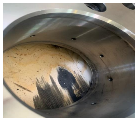
Fig. 7. Holes in the inner rim of the damper for supplying engine oil from the engine crankshaft
