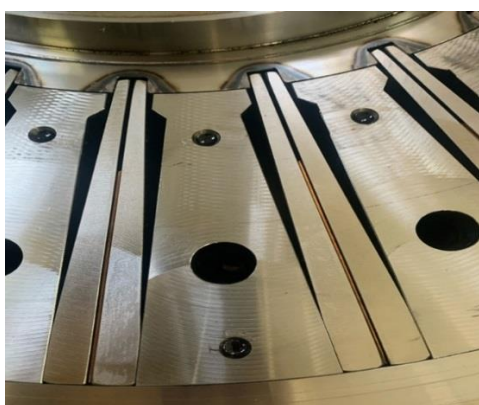
Fig. 6. The element of the intermediate insert with spring plates of the damper
